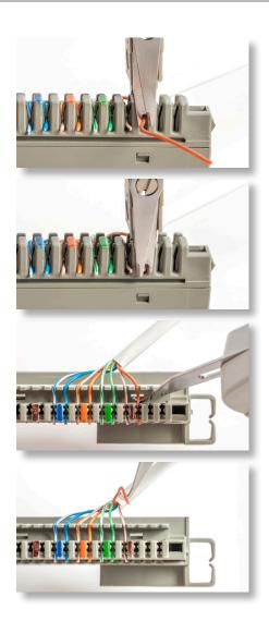
Designed to terminate and trim wires in Krone termination blocks, this punchdown tool is perfect for any telecom or data communications installer. This punchdown tool features the following:
